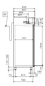
El = Electrical inlet (power) Refrigerant Inlet Refrigerant Outlet
